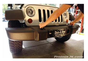
**10.** Using a phillips screwdriver, remove the 2 plastic screws securing the top plastic cover in place.
