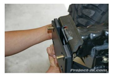
**16.** With the help of a friend, carefully place your new LoD Signature Series JK Front Shorty Winch Bumper on to the frame rails of your Jeep JK Wrangler and slide the mounting holes through the bolts you just installed. Reaching from the back, loosely secure it in place using the nuts provided.
