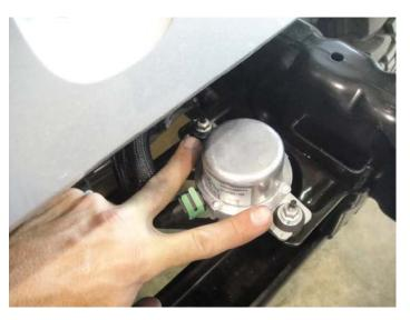
**4a.** With the switch out of the way cut the tab off that is closest to the front of the Jeep as shown in the photo.
