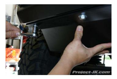
**33.** Secure the LoD Signature Series skid plate to the lower cross member of your Jeep JK Wrangler using the bolts and washers provided. You will need a 9/16" socket and wrench for this job.
