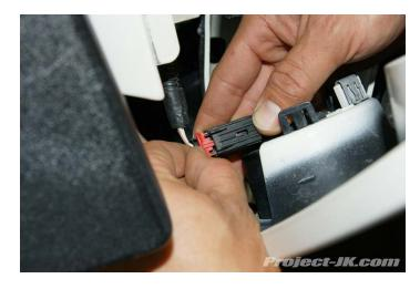
**26.** Squeeze the wiring harness plug and pull it out of your Jeep JK Wrangler's indicator light socket. You can now pull the grille off and set it aside for now.
