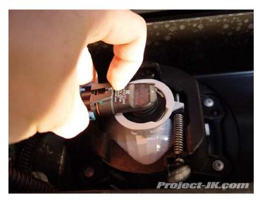
**5.** Using a pair of needle nose pliers, pry off all the fog light wiring harness connectors on the back of your Jeep JK Wrangler's front bumper.
