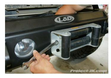
**29.** Carefully place your winch on top of the LoD Signature Series winch plate and then reinstall your Jeep JK Wrangler's grille as shown in this pic.
