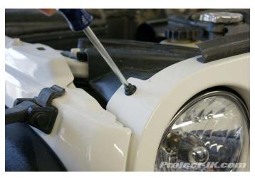
**24.** Once loose, the entire plastic screw and expansion sleeve should pull up and out of their mounting holes.
