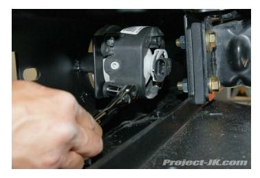
**23.** Using a phillips screwdriver, loosen the plastic retaining screws securing the top of your grille to your Jeep JK Wrangler.
