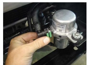
**3a.** Remove the two nuts that secure the switch. You can leave the switch wiring connected. Move the switch away from the mounting tab with studs.
