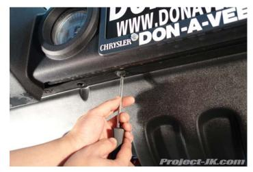
2. Once unscrewed, you should be able to pull out both the plastic screw and insert with little effort but if you find that your screws are just spinning (as several of mine did), you will need to wedge a flathead screwdriver or small pry bar between your JK's plastic bumper and air dam to help you force it out as shown in this photo.
