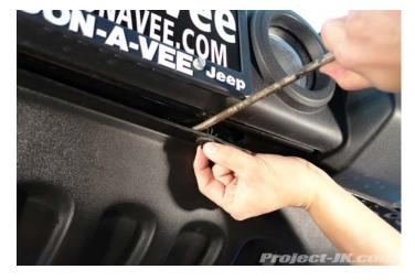
**3.** Now, climb under the front of your Jeep JK Wrangler and using a phillips screwdriver, remove the remaining 2 plastic screws securing the air dam to the lower cross member. As before, if these screws just spin in place, use a flathead screwdriver or small pry bar to help you force them out.
