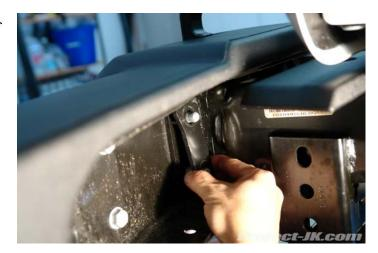
**9.** Carefully pull off your Jeep JK Wrangler's front bumper off the frame rails. If your JK came equipped with factory tow hooks, grab and use both of them to carefully pull your front bumper off the frame rails.
