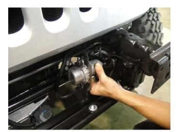
**6a.** With the bracket installed bolt the vacuum switch to the bracket as shown. The switch will be repositioned on its side in the new bracket.
