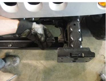
**5a.** Place the LoD relocation bracket up under the cross member as shown in the pic. Bolt the bracket on using the bolts provided with the kit. The bracket will mount directly up to existing holes so there is no drilling required.
