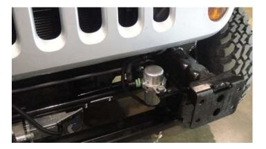
**2a.** Begin by removing the green clip that secures the vacuum line to the switch. Simply slide the clip down and pull the line off the switch.
