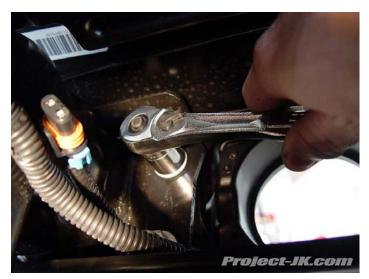
7. Using an 18mm socket, remove the 4 bumper mounting nuts (2 on each side) located next to the outside of your Jeep JK Wrangler's frame rails.
