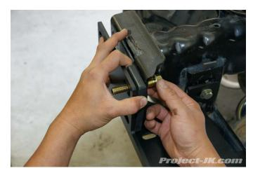
**15.** Repeat step #14 until all the steel spacers are installed in between the LoD Signature Series winch plate and frame rail bumper mount and that all the bolts are sticking through them as shown in this pic.
