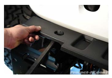
**11.** Again, if you find these screws to just spin in place, use a flathead screwdriver or small pry bar to help you lift up the cover off the frame rail and force the screw out.
