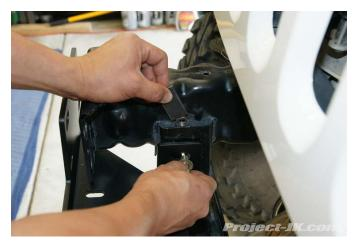
14. Slide one of the steel spacers in between the LoD Signature Series winch plate and frame rail bumper mount on your Jeep JK Wrangler. Then, insert the long bolts and washers provided with the bumper through the mounting holes and spacer as shown in this pic.
