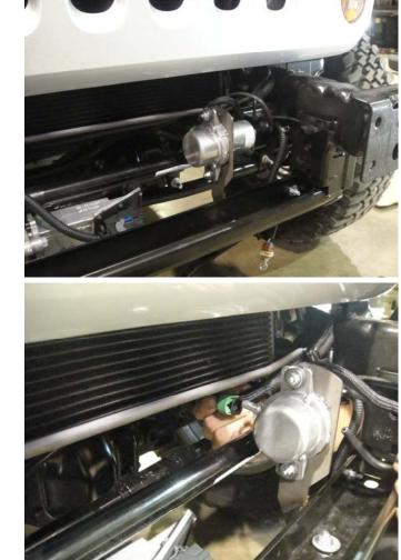
**7a.** Bolt the switch into place on the bracket.
