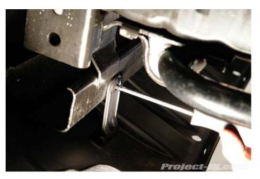
**4.** If your Jeep JK Wrangler came equipped with factory fog lights, climb under the front of your Jeep, look up behind the front bumper, locate the wiring harness plug, lift up the clip and then pull it off as shown in this photo.
