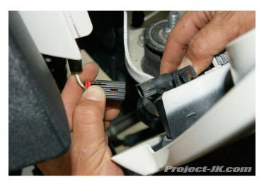
**27.** At this point you will need to extend your factory wiring harness to the fog lights since the fog lights are now relocated to a wider position than before. After lengthening the wiring plug your Jeep JK Wrangler's factory wiring harness back into the fog lights.
