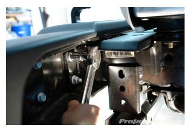
**8.** Remove the backing plates off the bumper mounting studs as shown in this photo.
