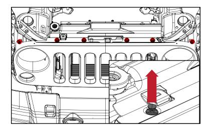
3. Pull bottom of grille away from vehicle to disengage metal clips on bottom rear of grille. Remove factory grille from vehicle.
