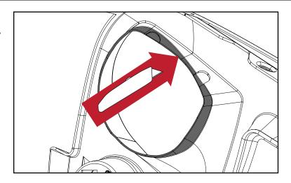
11. Install factory turn signal housing into Spartan Grille. Repeat for opposite side.
