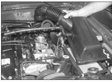
4. Unclip the air box lid, then, remove the upper intake assembly.
