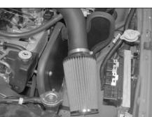
15. Install the K&N filtercharger onto the K&N intake tube as shown.
