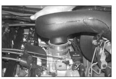
12. Install the K&N intake tube into the silicone hose on the throttle body.
