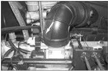
2. Loosen the hose clamp at the throttle body.
