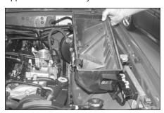
5. Loosen and remove the two bolts, and one nut to remove the lower air box assembly.
