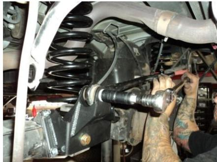
7. Reinstall trackbar into new higher location with factory bolt. (torque to factory specifications once vehicle is on ground and at ride height.)
