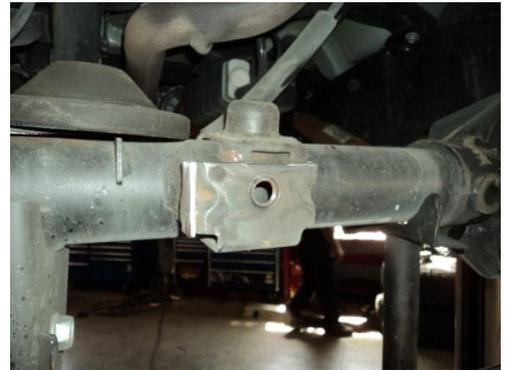
5. Install rear trackbar bracket as shown with supplied 9/16 bolt and U-bolts (make sure to use the locking nuts on the U-bolts).
