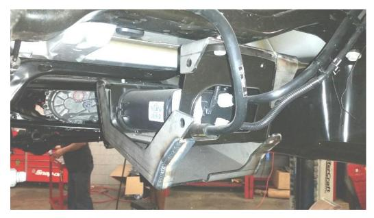
6. Install the supplied hardware tightly securing the EVO evap main skid to the EVO evap rear mount plate.
