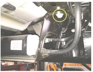
2. Loosen and remove the rear factory evap skid bolt completely.
