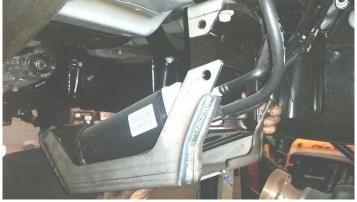
the rear of the factory evap skid can be nestled into the rear of the EVO Evap Main skid.
