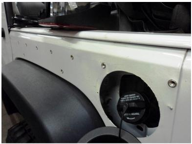
9. Install nutsets into drilled holes. Fully thread the long ¼" bolt with nut into the nutsert as seen in photo. With wrenches hold the bolt stationary and turn the nut 2 - 3 turns making sure that the nutsert does **NOT**
