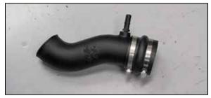
16. Install the provided hump coupler (5-576) all the way onto the K&N<sup>®</sup> intake tube but do not secure at this time.
