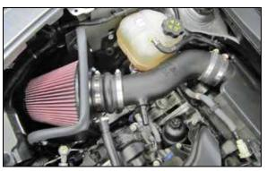
17. Install the K&N<sup>®</sup> intake tube into the coupler at the intake plenum and then slide the hump coupler onto the filter adapter. Adjust the intake tube for best fit and then secure with the provided hose
