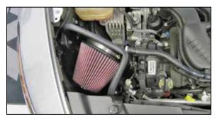
13. Install the heat shield assembly into the vehicle and secure with the hardware removed in step #6. **NOTE: Do not completely tighten at this time.**
