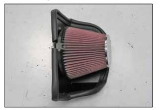
12. Install the K&N<sup>®</sup> air filter onto the filter adapter and secure with the provided hose clamp. NOTE: Drycharger<sup>®</sup> air filter wrap; part # RF-1048DK is available to purchase separately. To learn more about Drycharger<sup>®</sup> filter wraps or look up color availability please visit http://www.knfilters.com<sup>®</sup>. clamps and heat shield mounting hardware.
