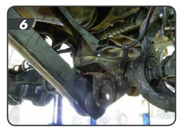
Lower the axle enough to remove the factory coil springs. Take care to ensure all hoses have adequate slack and the steering isn't binding. The drag link can be disconnected if necessary.
