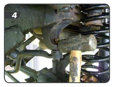
With the axle well supported, remove the shocks. Also remove the coil spring retainer located at the rear of the driver side coil mount.
