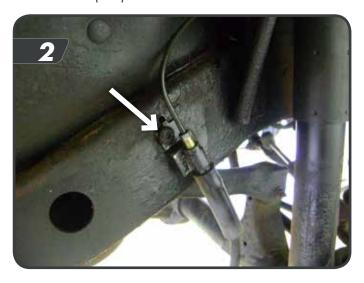
d. Disconnect the sway bar links from the axle and sway bar (18mm). Discard links and hardware. Note: If difficult to remove the sway bar link from the sway bar, an air chisel or pickle fork can be used.
