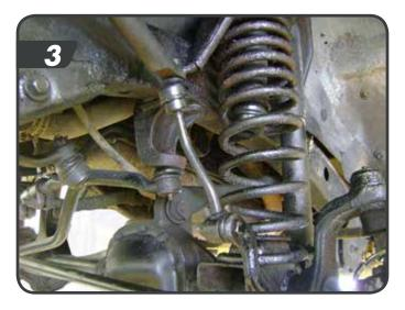
Disconnect the track bar from the frame rail bracket. Remove the cotter pin and nut (21mm) and thread it back on a few turns. Strike the track bar frame mount with a hammer to release the tapered seat. Remove the track bar.
