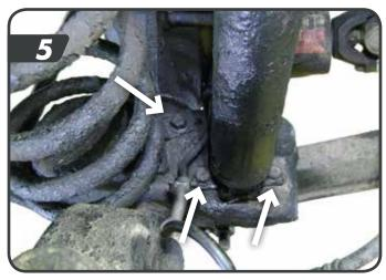
Remove the lower control arm to axle bolts.
