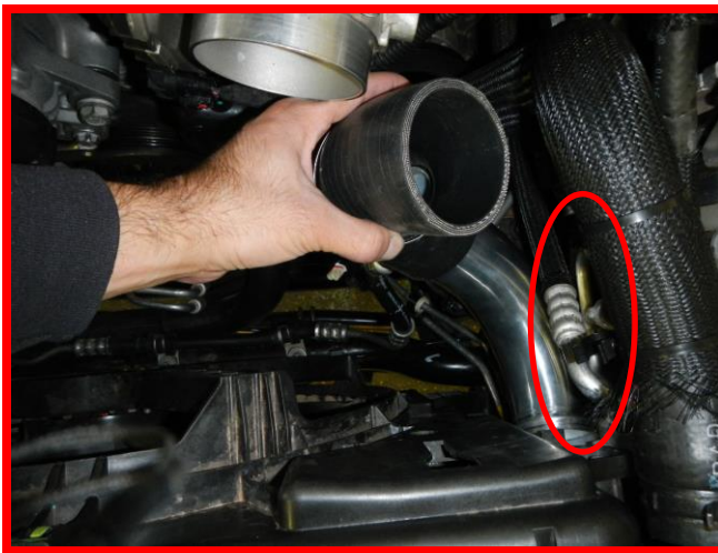
6) Bend AC line up slightly to make room for boost pipe, Install boost pipe leading to throttle body
