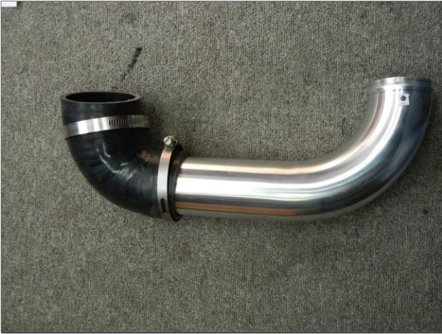
1) Assemble pipe loosely clamped
