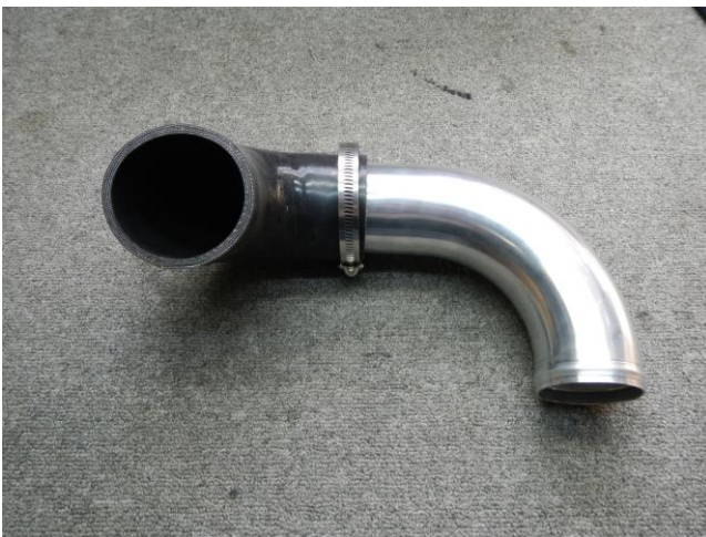
5) Assemble pipe loosely clamped
