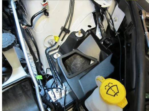
Air temp sensor (note tab direction)
