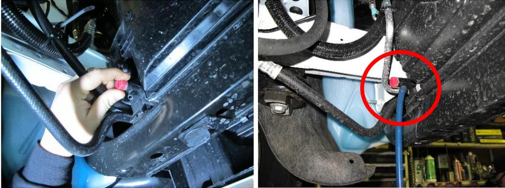
**Step (7): Remove upper coolant hose** from driver's side of radiator and cut approximately 2.25in off the radiator side of the hose or to the first bend FIG 1. This will make room for the supercharger installed in later steps. At this point please bend hose away from work area as per last picture. In later steps you will be reusing the factory clamp.
