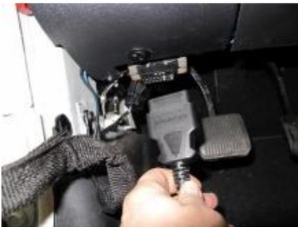
Before Installing tuner bring Diablo Tool to a PC with internet conductivity and plug in your Diablo with the supplied USB cable. Register tool and then update tool. This will insure newest tune will be uploaded to vehicle.
