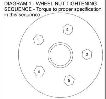
wheels are installed with good metal-to-metal contact. Improper installation could cause loosening of the wheel nuts. Never use oil or grease on lug studs or nuts.
