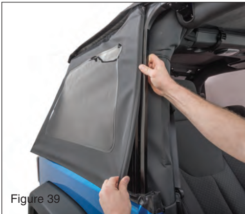
Begin to secure the windows by starting with the vertical lip on the side windows as shown. (see FIG 39)
