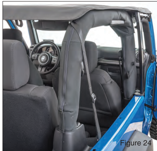
The top deck and the strap should reside at the approximate angles shown above. Final adjustments can be made later. (see FIG 24)
