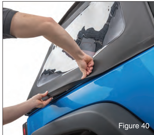
Slide lower window channel into body tub rail as shown. (see FIG 40)
