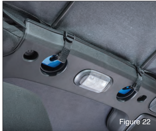
Wrap the two straps around the sound bar towards the rear and hook them as shown. Pull tightly to secure. (FIG 22)
