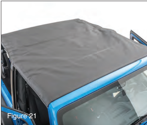
Unfold the top over rear of vehicle. (see FIG 21).
