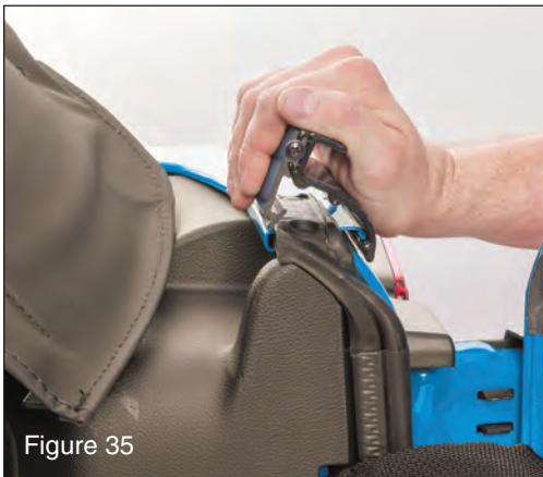
Place completed tailgate bar brackets onto rear body tub and carefully roll them forward in place. (see FIG 35)
