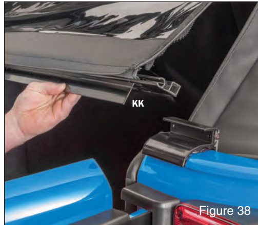
Slide the Rear Window Tailgate Bar (KK) onto the Rear Window as shown. Note orientation carefully. Insert the Tailgate Bar into the Tailgate Bar Retainers. (see FIG 38)
