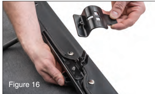
Unscrew and remove left and right header clamps from the windshield header channel. Set aside for step 20. (See FIG 16)
