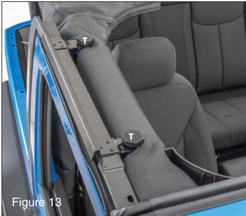
Insert the appropriate knobs (T) to secure the door surround. (See FIG 13) Repeat this procedure for the Left Side.
