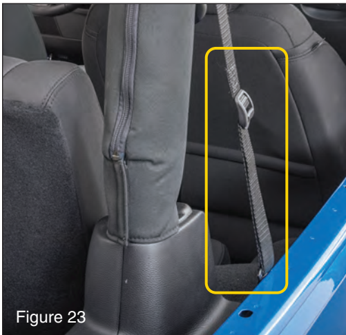
Locate the long strap on the rear of the top deck material. Pull strap down, and with buckle facing out, use the hook on the strap to grab and hold the body tub belt rail. Photo is zoomed in on the lower part of the strap. (see FIG 23)
