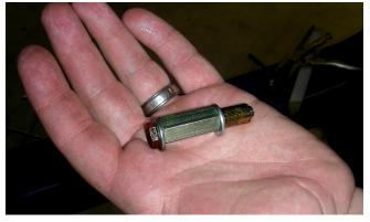
17. Use an open end wrench to hold the coupler nut stationary while turning the head of the bolt clockwise with a ratchet (or small impact wrench) and socket. As you turn the ratchet, the bolt will draw the far end of the nut-sert toward the inside of the sheet metal, gripping it with the knurled outside edge of the nut-sert as it deforms. Continue to turn the ratchet until the nut-sert is fully seated. DO NOT OVER-TIGHTEN as you can damage the nut-sert, or cause it to lose its grip.
