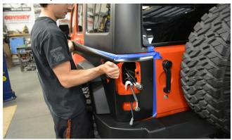
It is extremely important to ensure that the Crusher Corner is securely clamped into place, that it won't "walk" or loosen the clamps once you begin drilling.
