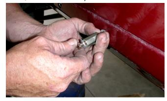
19. With the tool removed, inspect the nut-sert to make sure it is properly seated and that the surrounding sheet metal isn't excessively deformed. Note that some deformation of the sheet metal is normal, and that it will be covered by the part after installation.
