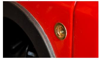
If you "spin" a nut-sert: That is, if it loses its grip due to over-tightening or improper installation, the quickest, easiest fix is to use a MIG welder to place a small tack weld at the edge of the nut-sert flange. Before applying the tack weld, sand or grind the paint from a very small area of the sheetmetal where the tack weld will be. Then insert a screw into the nut-sert to protect the threads from weld splatter. Only apply a very small tack or two, as you do not want to heat up and deform
