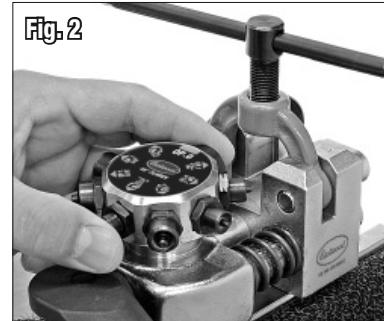
3. Place 11" foam-gripped handle into hole in lever base. Be sure to seat handle fully and snap groove into ball detent on side of hole.
