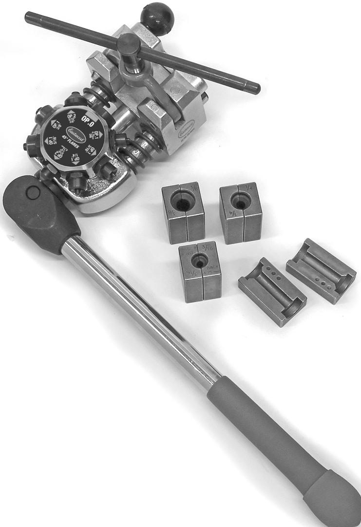
This **Eastwood Brake Tube Flaring Tool** will pay for itself with the first project, and it will give you peace of mind knowing that your brake flares are of OE-precision, quality, and safety. The tool mounts in your vise to help you easily form 45-degree single, double, and bubble flares in OE steel, stainless steel, and soft metal tubing for 3/16", 1/4", 5/16", 3/8", and 4.75mm-diameter lines.
