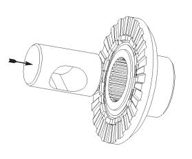
**15.** Insert the thrust block into the coupler that will go on the axle shaft opposite the ring gear.
