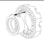
**19.** Insert driver/spacer as shown, making sure the spacer paddle is facing out towards you.
