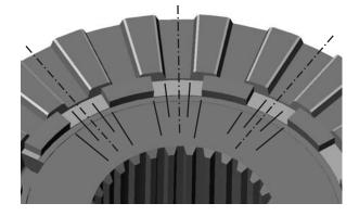
**13.** Apply wheel bearing grease to driver teeth and spacer.
