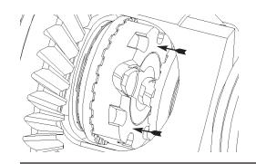
**20.** Verify spacer paddle is aligned with paddle opening in synchro ring and press driver/spacer down onto coupler. Driver teeth should be fully engaged all the way around.
