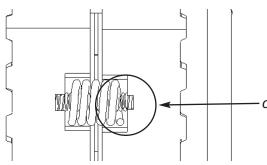
**28.** Visually inspect notches in spring slot to make sure inner spring is fully seated.
