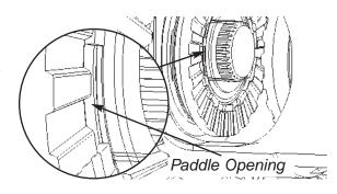
**18.** Insert an active spacer into a driver. Seat the spacer paddle at the paddle opening in driver (missing extended tooth).
