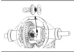
**10.** Remove passenger-side side gear/thrust block/thrust washer together. Retain thrust block.
