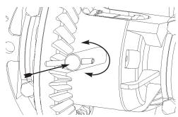
37. Drive roll-pin into case/shaft.
