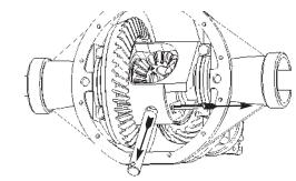
**8.** Remove the axle retaining bolts for the passenger side axle shaft located on the inside of the brake backing plate. Pull out passenger side axle shaft 2"-3". Slide thrust block to the right into the side gear.
