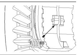
**31.** Visually inspect notches in spring slot to make sure inner spring is fully seated.
