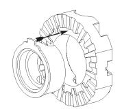
**21.** Insert the second active spacer into the second driver. Seat the spacer paddle at the paddle opening in driver (missing extended tooth).
