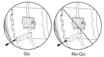
**32.** Check the gap between drivers using check block. The narrow side of the block should fit between drivers, but the wider side should not fit.
