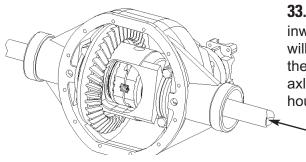
**33.** Push passenger side axle shaft inward through coupler as far as it will go. The axle shaft should push the thrust block against the opposite axle shaft. Bolt axle shaft back to housing.
