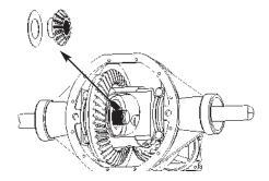
**11.** Remove remaining side gear and thrust washer.
