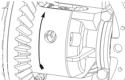
**36.** Using the roll-pin as a handle, insert the shaft into the differential. Press hard while twisting to pass shaft by springs.
