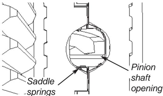
**34.** Keeping both drivers fully engaged, rotate both wheels back 1/4 turn to expose pinion shaft opening. Make sure saddle springs are all fully seated and the pinion shaft opening in the thrust block is aligned with the pinion shaft opening in the drivers.
