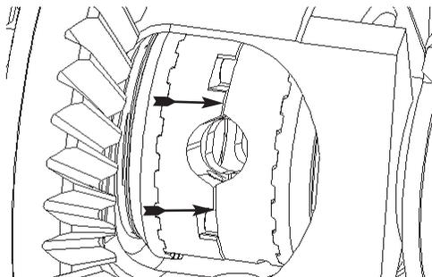
**25.** Wedge both drivers in engagement with couplers. Rotate driver's side wheel forward 1/4 turn to reveal spring slot.
