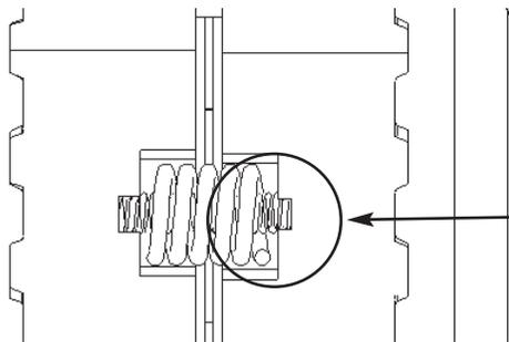
**28.** Visually inspect notches in spring slot to make sure inner spring is fully seated.
