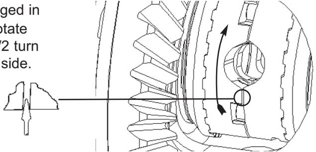
**30.** Compress inner spring and install the second spring assembly into the second spring slot.
