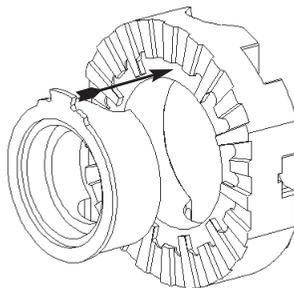
**19.** Insert driver/spacer as shown, making sure the spacer paddle is facing out towards you.
