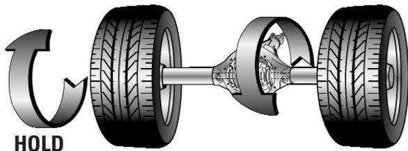
**41.** After sharply turning the passenger side wheel in the opposite direction (to disengage the unit), the wheel should rotate freely.
