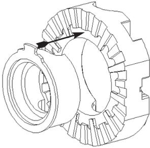
**21.** Insert the second active spacer into the second driver. Seat the spacer paddle at the paddle opening in driver (missing extended tooth).
