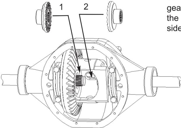
**17.** Make sure paddle opening (widest gap) in ring gear side synchro ring is facing out towards you.
