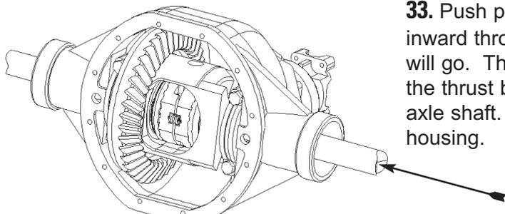
**33.** Push passenger side axle shaft inward through coupler as far as it will go. The axle shaft should push the thrust block against the opposite axle shaft. Bolt axle shaft back to housing.
