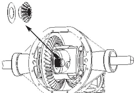
**11.** Remove remaining side gear and thrust washer.
