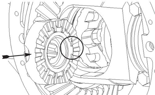
**24.** Verify spacer paddle is aligned with the paddle opening in synchro ring and press down on driver/spacer to seat on coupler; driver teeth should be fully engaged all the way around.
