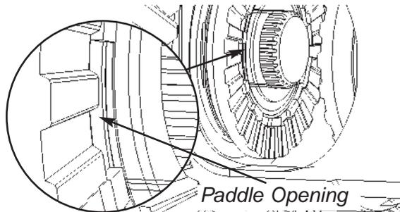
**18.** Insert an active spacer into a driver. Seat the spacer paddle at the paddle opening in driver (missing extended tooth).
