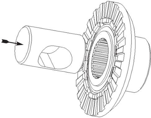
**16.** Insert the coupler into the ring gear side of the case first. Insert the coupler with thrust block into the side opposite the ring gear.
