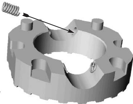
**15.** Insert the thrust block into the coupler that will go on the axle shaft opposite the ring gear.
