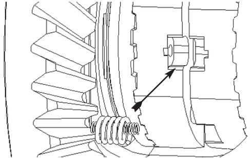
**31.** Visually inspect notches in spring slot to make sure inner spring is fully seated.
