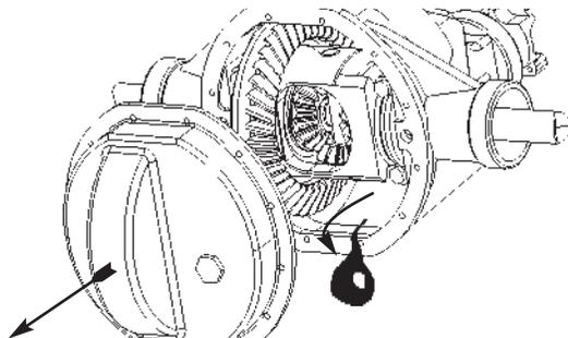
**7.** Expose pinion shaft; use a punch to drive out roll pin. Remove pinion shaft.
