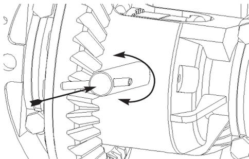
**37.** Drive roll-pin into case/shaft.
