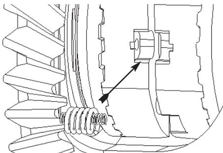
**27.** Compress inner spring and install spring assembly into spring slot.
