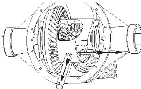
**8.** Remove the axle retaining bolts for the passenger side axle shaft located on the inside of the brake backing plate. Pull out passenger side axle shaft 2"-3". Slide thrust block to the right into the side gear.
