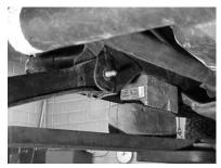
**Step 1:** Automatic transmission models require the removal of the factory transmission skid plate. Remove it first and re-install the nut on the driver's side, lower control arm bolt.
