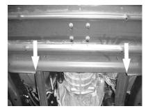
**Step 5:** Lift the engine skid plate and slide it over the threaded portion of the lower control arm bolt. Position the rear edge of the engine skid plate within the notched out area on the factory transfer case skid plate as indicated by the arrows in the picture to the right.
