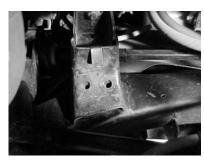
**Step 3:** Take the T-shaped plate with integral nuts and slide it into the driver's side motor mount through the top opening. Once the nuts can be seen through the two holes in the lower side of the motor mount, the tab may be folded over to hold the nuts in position. It is helpful to give the tab a slight arch before inserting it into the motor mount.
