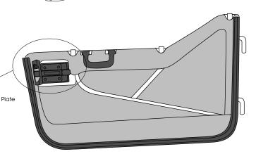
**Note:** If the lower door pivot does not provide enough adjustability for correct latch adjustment (the door does not latch properly), follow the instructions in the enclosed spacer kit.
