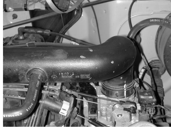
b) Remove the hose clamp securing the stock inlet tube to the throttle body.
