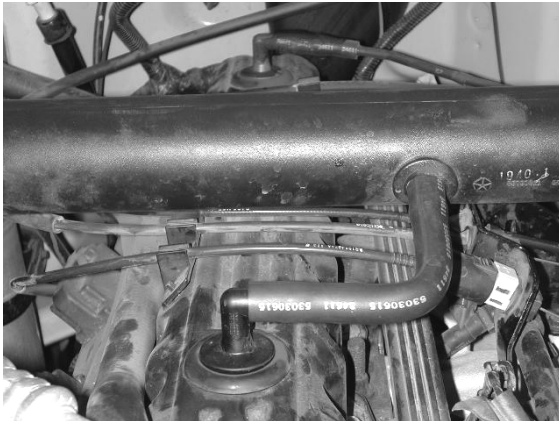
c) Remove the breather tube from the valve cover to the stock inlet tube.
