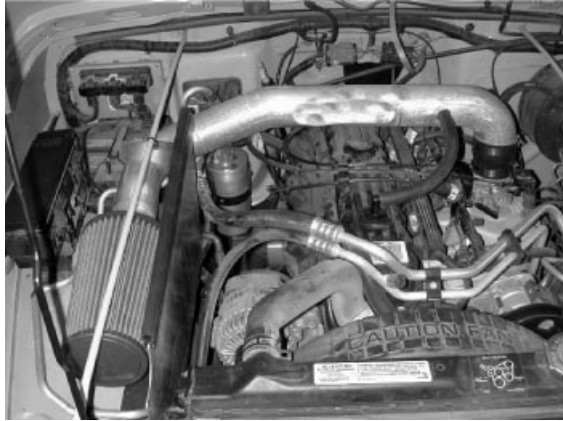
k) Intake installed on vehicle.
