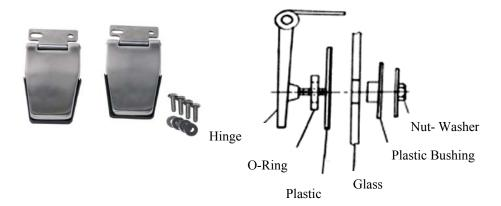
Install one side at a time beginning with the driver side. The driver side has the short stud on the inside. Remove the existing driver side at the glass area first then remove the two bolts holding the hinge to the hardtop.
