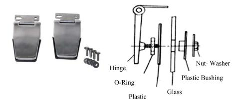
Install one side at a time beginning with the driver side. The driver side has the short stud on the inside. Remove the existing driver side at the glass area first then remove the two bolts holding the hinge to the hardtop.
