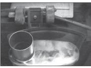
14.Install muffler with offset toward rear and inward.
