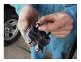
3/ Fit rockers to number one cylinder and tighten until all free play in pushrod is taken up and the pushrod cannot easily be rotated. This is the "zero free play" point.
