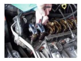
5/ More than 1 ½ turns will require installation of the silver spacer washers supplied in the kit under the mounting pedestals on the head side.
