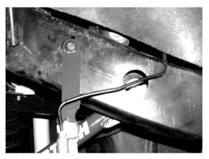
12. Locate the new Fabtech bump stop FT50027. Install into factory pocket by pushing bump stop in until fully seated. SEE PHOTO BELOW.
