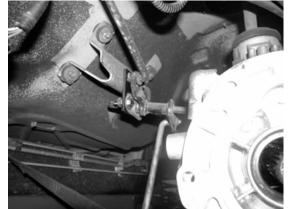
Locate the Fabtech transmission crossmember spacers FT50024. Using the correct supplied bolts and washers for your year Jeep, <sup>1</sup>/<sub>2</sub>" x 2 <sup>3</sup>/<sub>4</sub>"(1997-2002) or 12mm-1.5 x 69.5mm (2003) reattach factory crossmember to the truck with the Fabtech spacer between the frame and the crossmember. Torque bolts to 85 ft lbs. SEE PHOTO BELOW.
