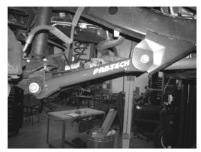
10. If installing Fabtech's optional upper link arm kit, install front upper at this time. See instructions included in Fabtech's upper link arm kit.
