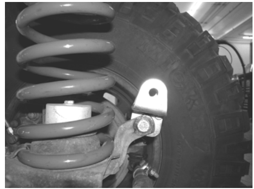
Note position of bracket, slight tilt forward
