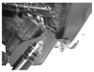
8. Torque the steering box bolt to 70 Ft. Lbs. Torque the bumper bolt to 80 Ft Lbs. Torque the inner bolt 30 Ft. Lbs.
