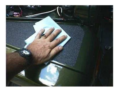
Rub <u>from the center of the Protector out toward the edges</u>. This will help eliminate air pockets.
