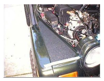
When you are satisfied with the alignment and installation, use a clean dry paper towel or the Protector Backing Paper and <u>thoroughly rub down the enter Protector</u> to finish adhesion.
