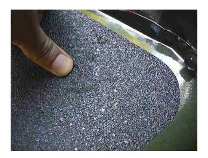
Press a Philips Head screwdriver into each indentation to open up the five (5) holes in the top of the fender needed to mount the latch and bumper.
