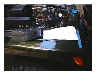
Continue to lay the front half of the Protector down onto the fender. **<u>DO NOT** rub down yet</u>. If the location is off you can lift the protector and re-align it.
