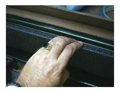
Then press the vertical surface of the protector down against the Sill using the backside of your finger to work out any air pockets.
