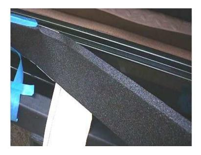
Carefully seat the Sill Protector to the Sill at the Bend.
