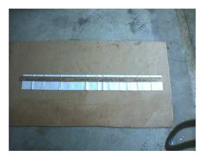
Form (bend) the Sill Protector up to form an angle close to 90 degrees. The angle does not have to be a perfect, but do take care to make the bend in a straight line across the entire protector.
