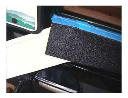
Continue to lay the left side of the Protector down along the bent edge onto the Tailgate Sill. **DO NOT** rub down yet. If the location is off you can lift the protector and re-align it.
