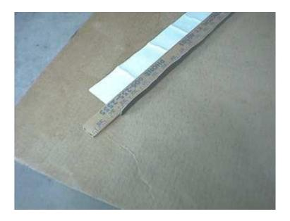
Place the Tailgate Sill Protector on the Tailgate Sill and position it where you want it. Pay particular attention to the area where the protector bends into the rear door jam.
