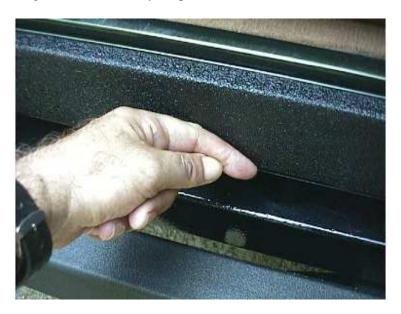
Finally using the Tailgate Sill Protector Backing Paper or a clean paper towel <u>thoroughly</u> <u>rub down the enter Protector</u> for finish adhesion.
