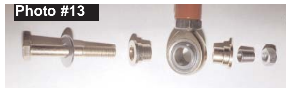
5/16" x 3/4" thread cutter flange bolt.
