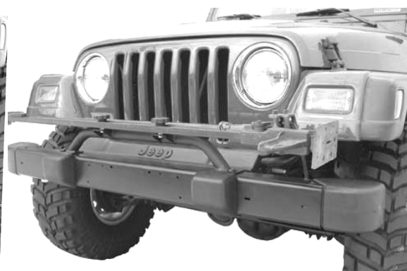
180- Auxiliary Bar with Hi-lift jack mounted on OEM bumper Using 181-Hi-Lift jack mounting kit.
