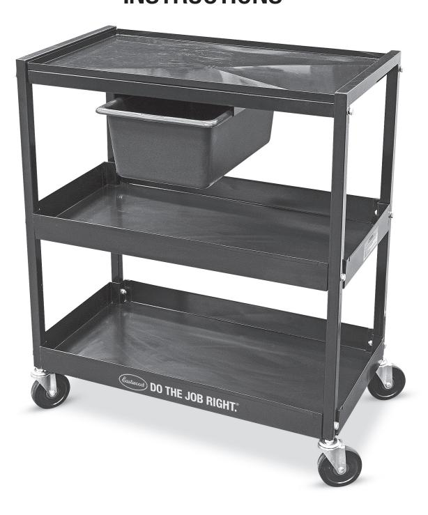
The **EASTWOOD TEAR DOWN TABLE** features a spacious, powder coated, steel work surface with integral drain and a solvent-resistant polyethylene Fluid Containment Basin. The heavy, all steel support structure and 4" swivel casters support up to a total loaded weight of 250 lbs. [113kg.] yet is completely portable for rolling to the job and between project storage.
