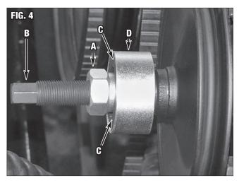
Slide the Hub Remover Shell [D] over the mated Hub Remover Jaws [C], Remover/Installer flange and pulley hub to tie everything together (FIGS 4 & 5).
