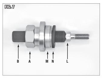
• Thread the assembly into the end of the pulley shaft with the Thrust Bearing against the pulley hub face (Fig 8) and tighten with a 1" wrench to draw the pulley onto the shaft.
