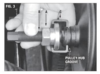
• Place the 2 identical halves of the Hub Remover Jaws [C] around the hub of the pump pulley and Remover/Installer [A] flange (FIG 4). NOTE: The larger I.D. of the Jaws should be toward the Remover/Installer as shown in (FIG 3).
