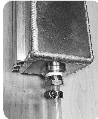
Tubing attached to bottom of Overflow tank
