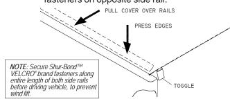
**STEP 8:** To release cover, pull back on toggle. Roll cover toward cab to open. For best results, leave cover fastened to side rails while opening.
