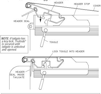
NOTE: In cold weather conditions or with some accessories, it may be preferable to close the cover before closing the tailgate. Header seal may be placed across top of tailgate if preferred.
