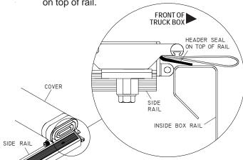
**STEP 5:** Slide header guides into side rail flanges on each side of header. Tighten bolts securely.
