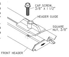
**STEP 4:** Set cover assembly behind cab with header seal on top of rail.
