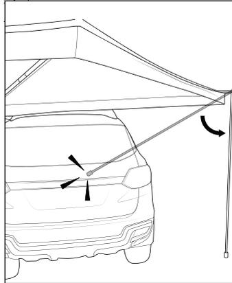
Be aware on some vehicles the 4th support can hit the rear of the vehicle when dropped down. Simply undo the tension strap, drop the support, then re-attach the retention strap.
