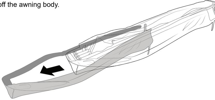
**3c** Slide the new bag in as shown. Be sure correct orientation is used. The matte finish of the PVC bag faces the outside. Replace the plastic plugs with those provided in the new bag kit.
