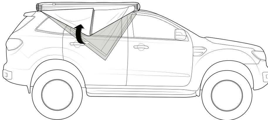
2. Roll the material from the front edge back up into its original setting.
