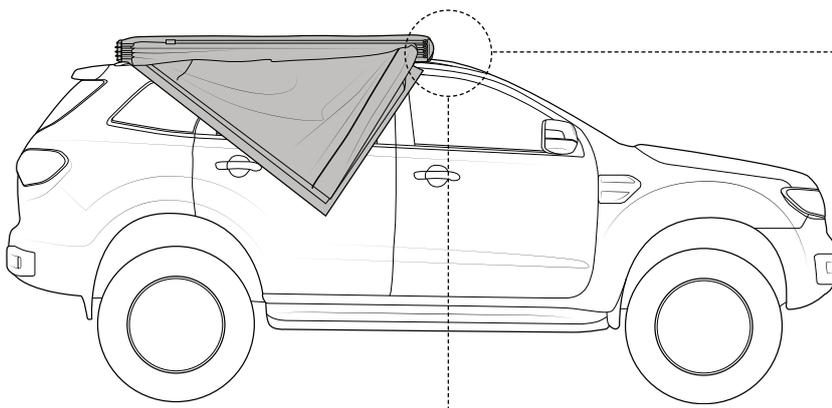
**X** (fig A) If the arm is off centre as shown, the magnet in the end cap will not secure the arm in place properly.
