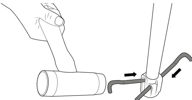
Leave a small gap to allow pegs to be removed easily.
