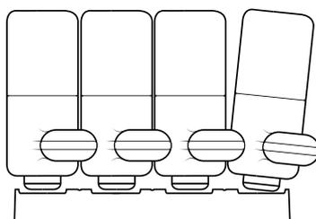
(fig B) Loosen the screw behind the drop down hinge, adjust the arm rotation and re-tighten the screw.
