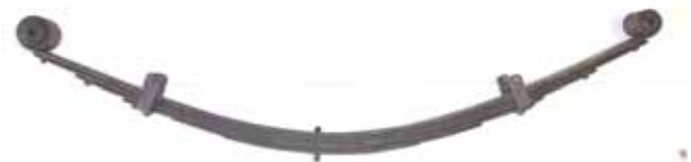
< FRAME END (LARGE BUSHING) – PHOTO 4 – SHACKLE END >
