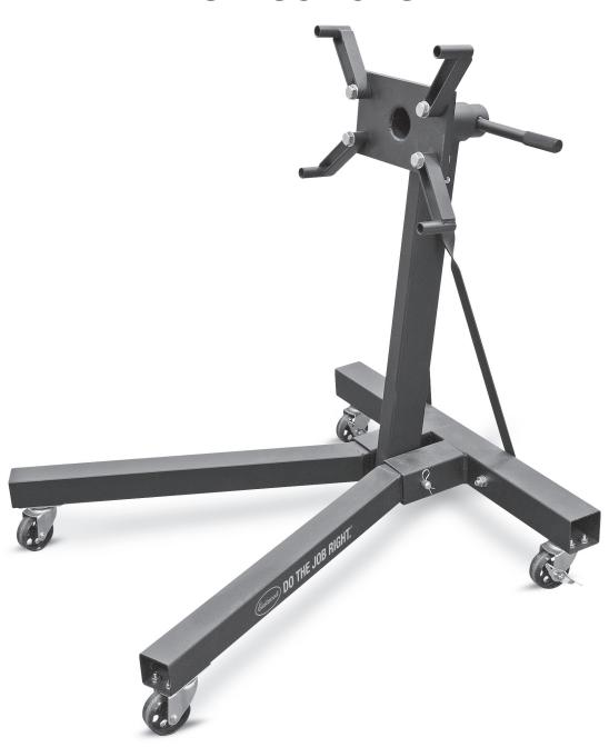
The **EASTWOOD 1200 LB ENGINE STAND** features an efficient folding design to minimize storage space when not in use. A wide footprint provides a solid, stable base. Features a rotatable Spindle with 6 locking positions. Steel, ball bearing Locking Swivel Casters and a rugged steel Frame will support up to a total loaded weight of 1200 lbs. [544 kg.] yet is completely portable for use as a work stand or for long-term storage of engines and transmissions.
