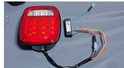
Step 6: Tap into existing wiring harness:
