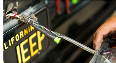
Step 3: Disconnect the tail light harness.
