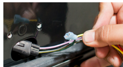
Step 9: Crimping completed. Feed harness into chassis.
