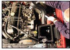
Loosen the 3 nuts that hold the stock air. box to the fender well of the vehicle.
