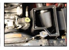
Attach the air box lid to the air box. Installation is complete. Check all mounting points for tightness and reconnect the battery
