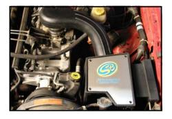
Bolt the S&B cold air box to the fender wall. "Place the stock air box grommets underneath the air box". Use the stock
