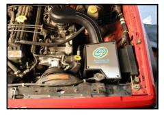
Unbolt the stock air box and remove
