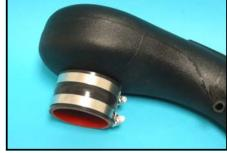
Install the S&B cold air tube thru the S&B cold air box and onto the throttle body
