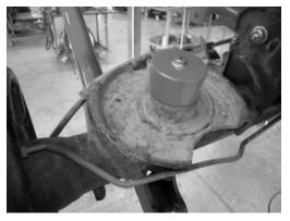
51. Locate the previously remove brake line and e-brake cable from the upper link arm. Reattach to the Fabtech link arms using factory hardware on the passenger side and the supplied 5/16" bolt, nut, and washer on the driver side. SEE PHOTO BELOW.
