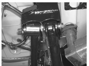
49. Locate the upper bump stop cup, remove and discard bolt. Locate the bump stop drop spacer FT50062 using the supplied 10mm-1.5mm x 105mm bolt and washer install the spacer between the bump stop cup and upper coil seat. Install the Fabtech upper bump stop FT50027, into the stock location. SEE PHOTO BELOW.
