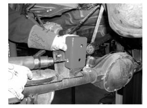
59. Locate the Fabtech upper frame Trac bar bracket FT50054. Using the supplied <sup>1</sup>/<sub>2</sub>" x 1 <sup>1</sup>/<sub>4</sub>" bolt, and washer and <sup>1</sup>/<sub>2</sub>" x 3 <sup>1</sup>/<sub>2</sub>" bolt, nut, and washer attach the bracket to the frame. Torque both bolts to 75 ft. lbs. SEE PHOTO BELOW.
