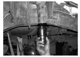
20. Locate the new Fabtech lower Aluminum bump stop FT50052. Using a drill, drill a 5/16" hole through the center of the lower coil spring mount. Using the supplied 5/16" x 2 <sup>1</sup>/<sub>2</sub>" bolt, nut, and washer attach to the lower coil spring mount. SEE PHOTO BELOW.
