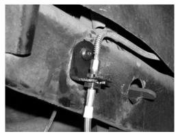
18. Locate the supplied brake line retaining spring and Adel clamp. Using a drill, drill a guide hole directly below the brake line bracket on the frame. Attach the spring to the frame using the supplied 5/16" self tapping screw. Attach the other end on the spring to the brake line using the supplied Adel clamp and ¼" bolt, nut, and washer. SEE PHOTO BELOW.
