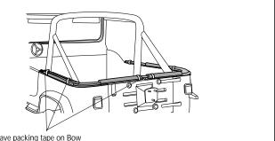
Leave packing tape on Bow Assemblies until front holes of Bow Mounts are secure
