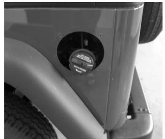
Figure #1 – Remove Gas Tank Outer Flange
