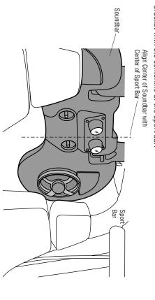
remove the vehicle top. Note: The soundbar may be installed with the top on the vehicle, but for easier installation
