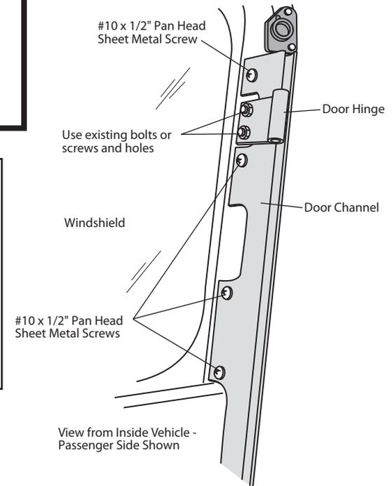
**NOTE** If your vehicle has this type of Door Hinge, replace it with one from the parts kit.
