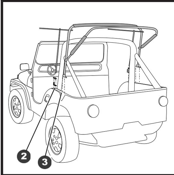
**CAUTION** When drilling in the top edge of the vehicle body, check underneath for wiring for the rear lights. Pull the wiring out of the way before drilling.
