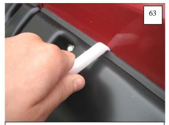
Using curved end of supplied Edge Trim Tool, seat top edge of edge trim first by hooking curved end under top edge at one open end and slide over entire top edge to the other end.
