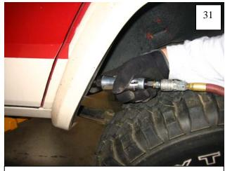
Using a 10mm socket, remove the factory fastener located inside the front of the wheel well.
