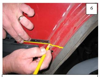
Starting at the bottom of the headlight bezel, measure in 5" and mark a line on the fender.
