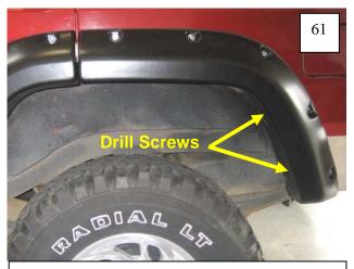
Optional: There are extra drill screws supplied in the kit. If desired, further secure the rear of the rear flare using drill screws. Place drill screw on part and drill into sheet metal.
