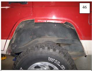
The fender should look like this. Some additional grinding may be needed. Optional: use caulking to seal all cut edges and seams.
