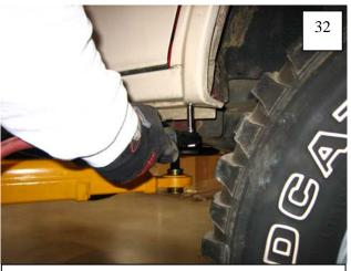
Using a 7mm socket, remove the lower front factory fastener.
