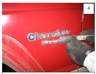
Apply adhesive remover to the Cherokee emblem for ease of removal. Using a putty knife, carefully remove the Cherokee emblem, taking caution not to scratch the paint.
