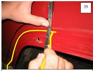
Make a vertical line 1" back from door edge, intersecting with line made in Step 34.
