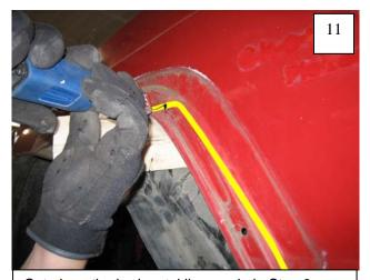
Cut along the horizontal line made in Step 9.
