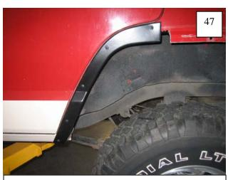
Open door. Install cover piece over "dog leg" using five supplied drill screws. Place drill screw in indent in part and drill into sheet metal. NOTE: Some trimming may be required.
