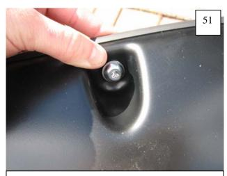
Insert screw and washer through each pocket in flare.
