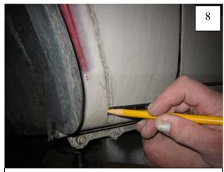
Starting at the edge of the door seam, measure in (towards fender well opening) 5-1/4" and make a mark.
