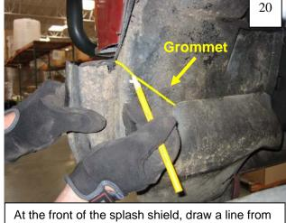
At the front of the splash shield, draw a line from the area cut in Step 19 down to the plastic grommet, taking care not to cut through the grommet. Trim on this line.
