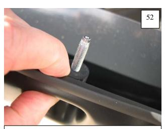
Place a 3/8" thick rubber spacer on each screw from the backside of the pocket. Threads must protrude through spacer for proper attachment of flare. All spacers must be installed prior to installation on fender.
