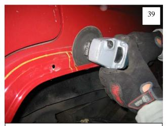
Starting at top of fender, cut along lines using a reciprocating saw or cut-off wheel.
