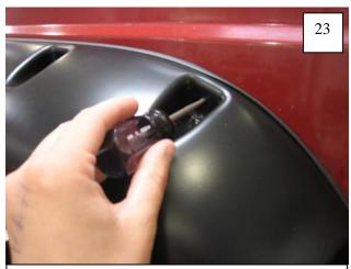
Hold the Front Flare in place on the fender, pressing firmly. Using the holes in the part as a guide, mark hole locations on fender (9 places).
