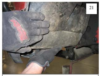
Fold the remaining flap under the bumper.
