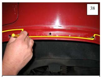
Measure up 3/8" from edge of fender well, intersecting with line made in Step 35 and mark a line continuing along edge of fender until intersecting with line made in Step 37.
