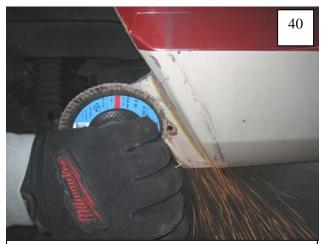
Along rear fender well edge, take care not to cut through weld seam. Cut close to seam, then grind back.
