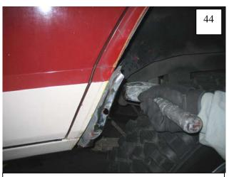
Using a hammer or mallet, pound the inner sheet metal layer over the seam.
