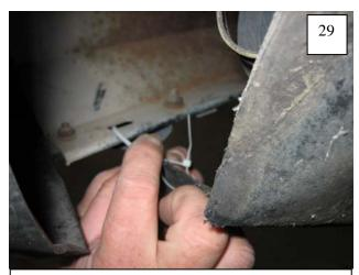
Optional: To secure splash shield, drill a hole and use a zip tie to attach it to the bumper.
