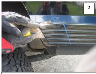
Use a putty knife to separate the factory trim from the fender, stopping at line made in Step 2.
