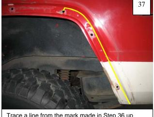
Trace a line from the mark made in Step 36 up along the contour to the third factory hole (counting from bottom rear). Drop line down to intersect hole.
