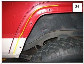
Follow contour up to 1" past the door edge, maintaining a distance of 2" from edge of wheel well.
