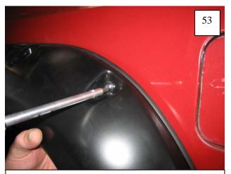
Start each screw with supplied Torx bit in each pocket but do not tighten until all screws have been started. Over-tightening screws may cause them to strip! Use a Torque setting of 90 inch/ounces.
