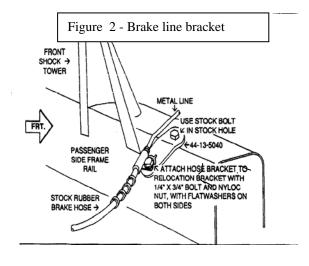
Assemble as shown with brake line bracket mounted to the frame in the stock brake line location. Pull the steel line out from the frame and bolt it in the other hole on the bracket.
