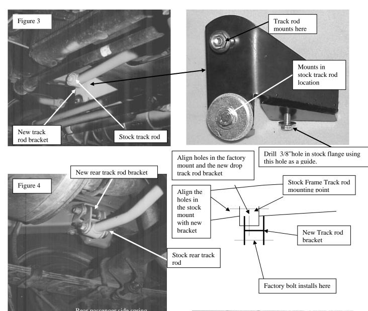
Remove the brake clip at this location. This will allow the steel line to be pulled out from the frame mount. Install the bracket as shown with a bolt through the small hole of the bracket and stock mounting point.
