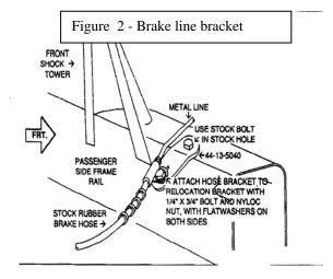
Assemble as shown with brake line bracket mounted to the frame in the stock brake line location. Pull the steel line out from the frame and bolt it in the other hole on the bracket.
