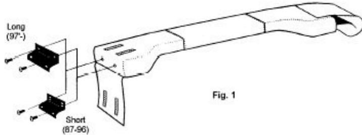
NOTE: The short bracket has 2 sets of holes to mount to the Sound Bar. These allow the height of the Sound Bar to be adjusted.
