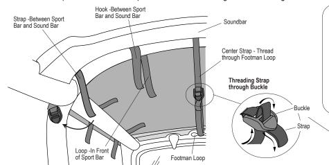
Note: Some soundbars fit extremely tight against the sport bar preventing the buckles easy access to the straps. If this is the case, the soundbar must be moved slightly rearward. The distance will vary on each vehicle.
