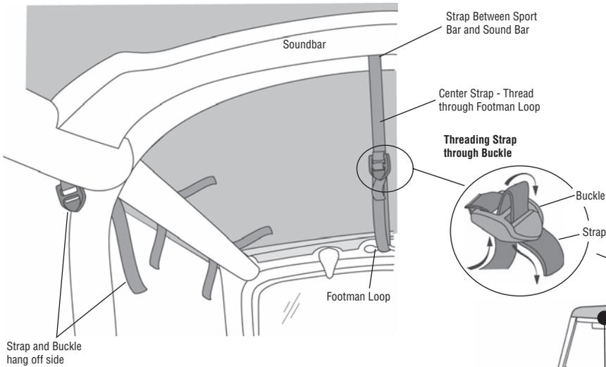
**Note: Some soundbars fit extremely tight against the sport bar preventing the buckles easy access to the straps. If this is the case, the soundbar must be moved slightly rearward. The distance will vary on each vehicle.**
